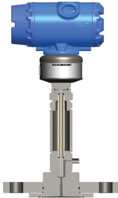
Figure 6. In some hot applications, it is required to add additional separation from the process heat to the transmitter. This shows an example cut-away view where the oil fill lines extend to the sensor and protect the temperature of the transmitter
