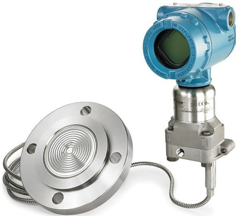
Figure 3: This remote seal configuration can be mounted in direct contact with the process fluid, and the pressure transmitted via an inert fluid to the pressure sensor
