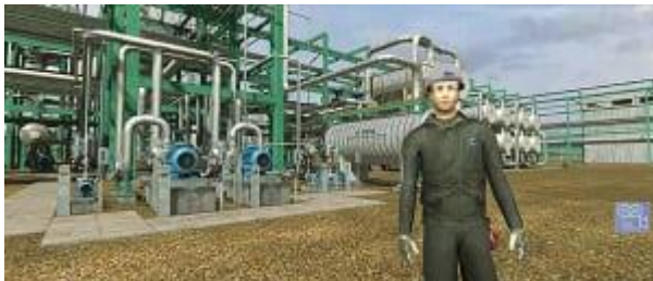
Figure 3. This virtual reality environment for an IGCC plant offers realistic training opportunities
